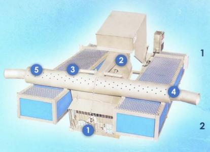
Impeller. Water is drawn from below the surface into the bar-screened area. Depth of water draw can be adjusted. Smaller units draw from the front of the impeller, the largest unit draws from the front and the rear. The impeller can pump up to 1.5-inch-diameter solids. Water is fed into the large 305-L stainless steel discharge manifold pipe.
